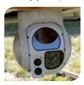
The **LIAZ Gimbal** is the UVA's key component. It is composed of a gyro-stabilized suspended hinge and an electro-optical sensor that enables the **SkySpotter 151** to perform a wide range of real-time monitoring tasks: object detection and tracking, object search and localization, image capture and transmission in visible or infrared spectrum, nightvision and precise focus on the tracked object.
