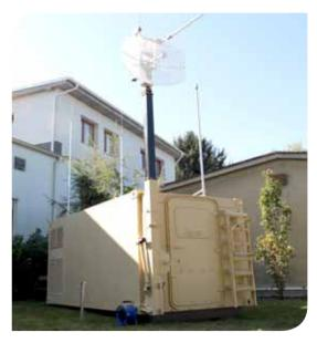
The **LIAZ GCS** ground control station remotely controls the aircraft and provides control and data communication with attached equipment (payloads).
